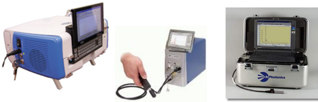
Figure 10. Portable Raman spectroscopic devices. (Left) MiniRam, (center) MiniRam II (B&W Tec), and (right) InPhotote (InPhotonics)
